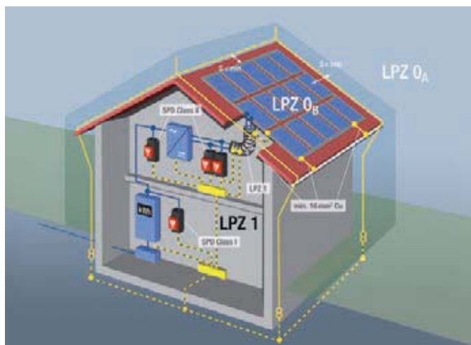
Figure 5: Building installation with external lightning protection, not in compliance with air termination distances
