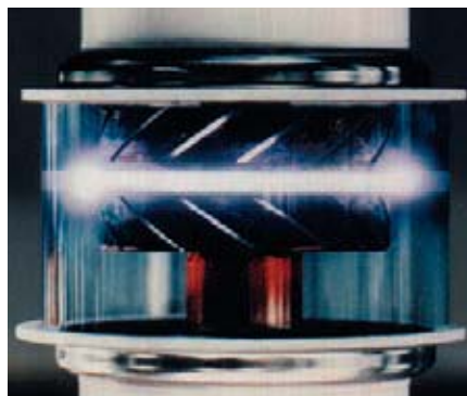
Electric arc in a 10 kV switch while being switched off
