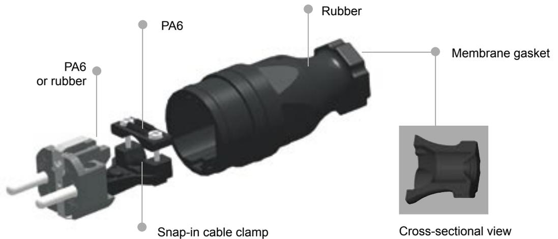
Max. 3G2,5 mm<sup>2</sup> rubber-sheathed flexible cable
