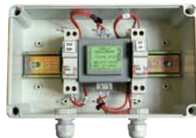
TBExx Waterproof power supply boxes IP67 M2 220-240/24 Volts AC With primary & secondary protection fuses. To be placed in spy holes or in the lighting poles of public installations.
