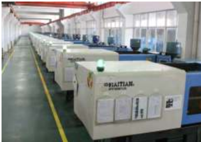
Precise plastic injection machines
