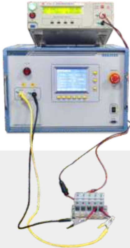
Power frequency withstand voltage/ impulse withstand voltage test of din rail terminal blocks
