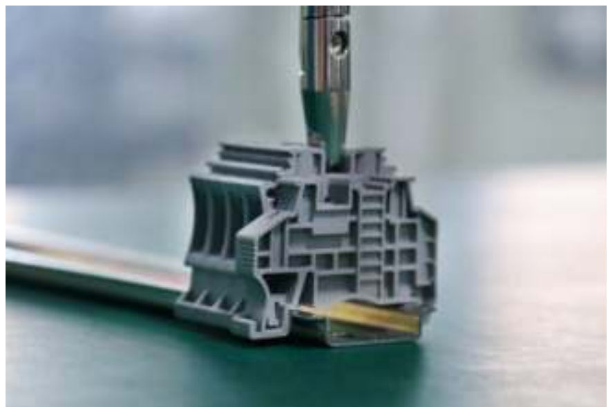
Din Rail Terminal Blocks Touch Protection Test
