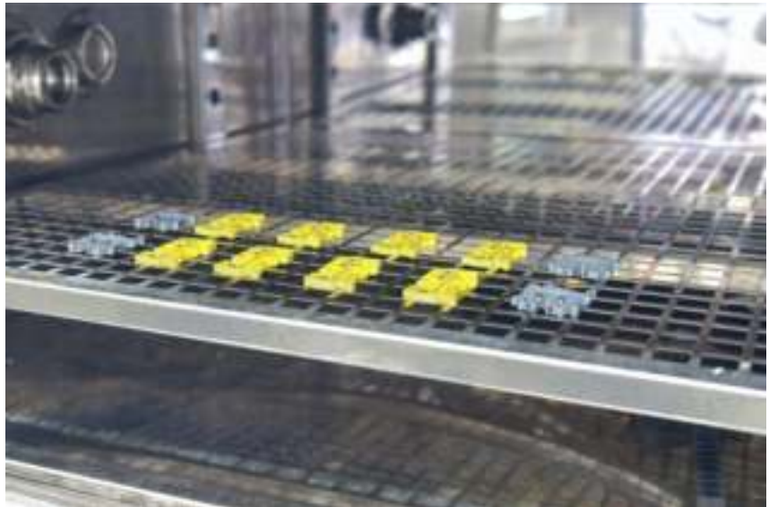
Din Rail Terminal Blocks Temperature Cycling Test
