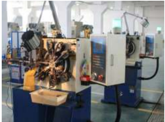
Automatic (spring) forming machines
