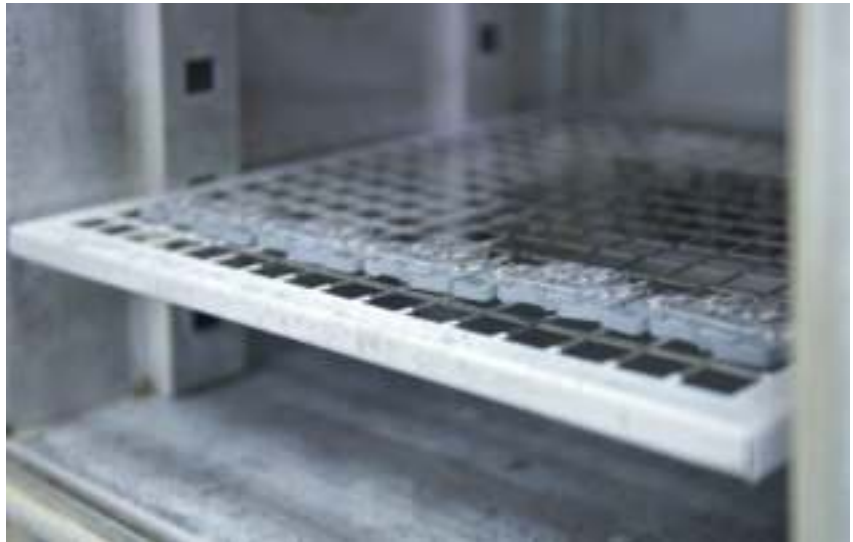
Din Rail Terminal Blocks Temperature Cycling Test
