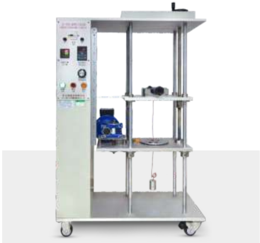
Din Rail Terminal Blocks Rotational Pull Test
