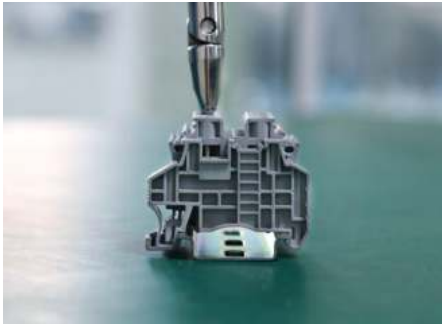
Din Rail Terminal Blocks Touch Protection Test
