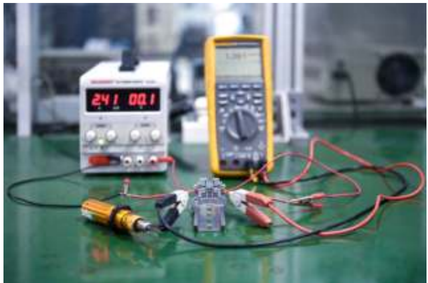
Din Rail Terminal Blocks Voltage-drop Test
