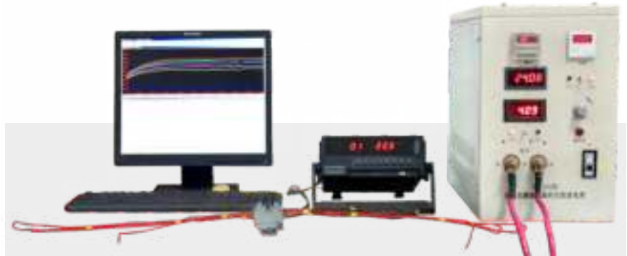
Din Rail Terminal Blocks Temperature-rise Test
