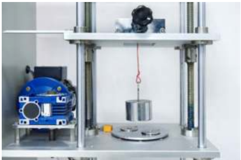
Din Rail Terminal Blocks Static Pull Test
